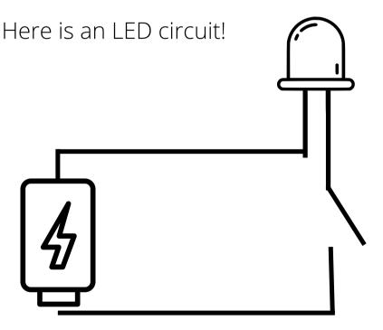
When these two wires connect, the circuit will close and the LED turns on. While they are separated, charge cannot flow and the LED is off. This creates a natural on/off switch for the circuit.
