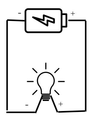
A circuit is a closed loop where charge can flow, a complete path of conductors with a power source and something to be powered. A power source, like a battery, sends a positive charge through conductors to reach the load, or the thing that uses the power. Negative charge then returns to the power source. Power sources can be batteries and the load is often lights or a motor of some kind.
